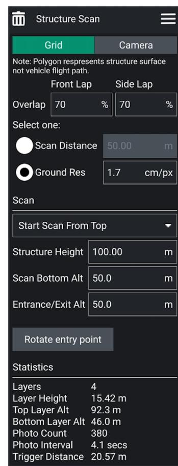
**Rotate entry point:** Move the start/finish point to the next vertex/position on the flight path.
